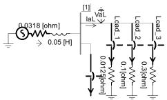
Fig. 6: A single line diagram of a simplified power system model used in the PSCAD Simulation.
