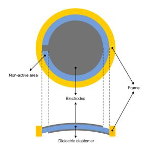
Figure 2. Construction of tactile stimulator
