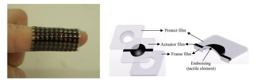
Figure 6. Wearable tactile display
