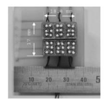
Figure 5. Braille tablet by assembling six modules of Braille cells
