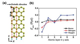
**Fig. 1** (a) Scheme of  $3 \times 1 \times 1$  eight-layer ZGNR supercell with a single edge H-saturated. The unit cell is indicated by the red dashed line; (b) plot of substitution energies of heteroatoms on carbon atoms at different layers as indicated by the number in (a).
