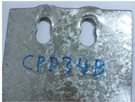
(a) Shear out failure
