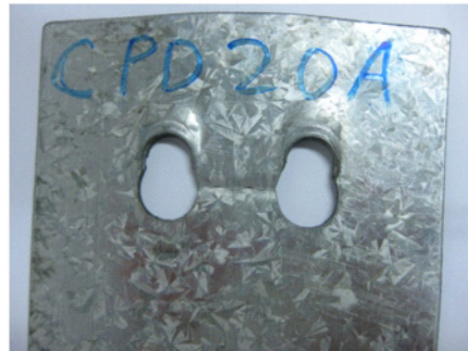
(c) Block shear failure
