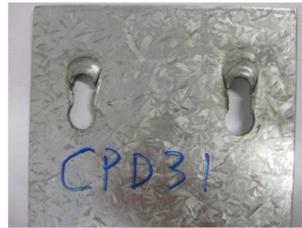
(b) Bearing failure
