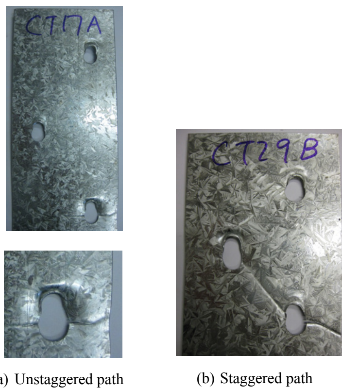
Figure 7 Failure paths of double shear 1.5 mm specimens
