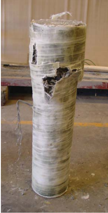
Figure 4 – Column G0 – Internal Reinforcement with Three Layers E-Glass – e=0\text{mm}
