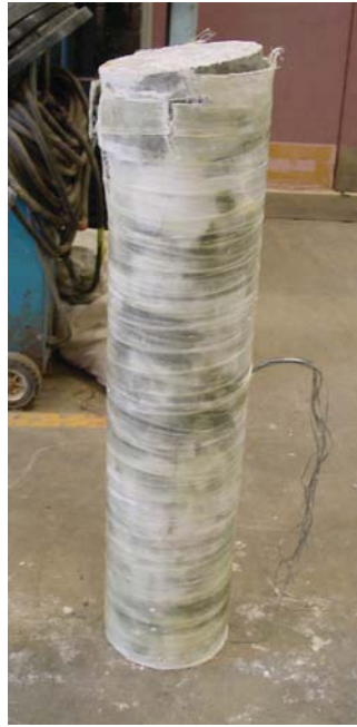
Figure 10 – Column G50 – Internally reinforced with Three Layers E-Glass – e=50\text{mm}
