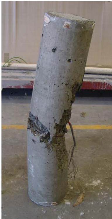
Figure 5 – Column N25 – Internal Reinforcement Only – e=25\text{mm}
