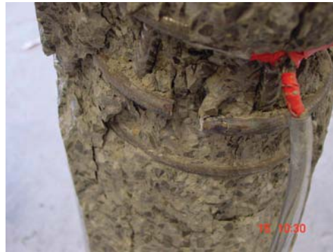
Figure 5 – Column N25 – Internal Reinforcement Only – e=25\text{mm}
