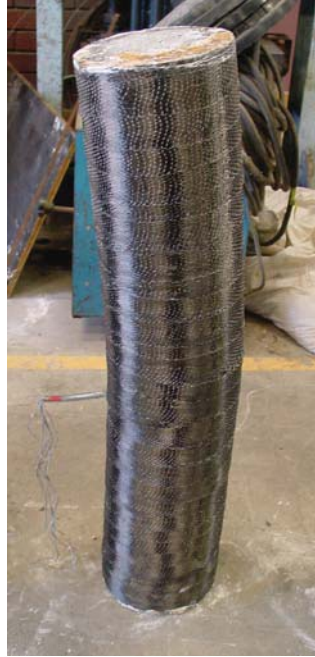
Figure 9 – Column C50 – Internal Reinforcement with Three Layers Carbon – 50mm
