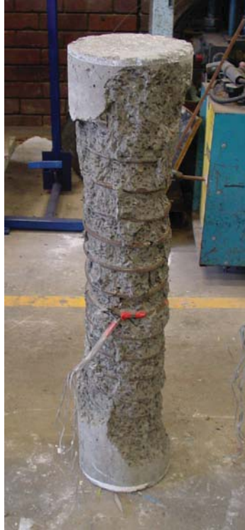
Figure 8 – Column N50 – Internal Reinforcement Only – e=50\text{mm}
