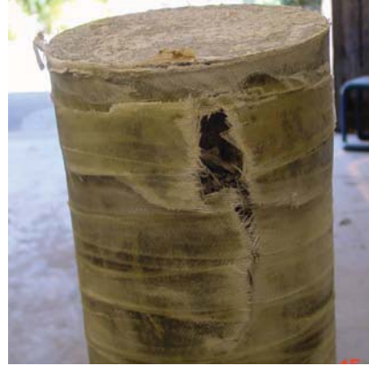
Figure 10 – Column G50 – Internally reinforced with Three Layers E-Glass – e=50\text{mm}
