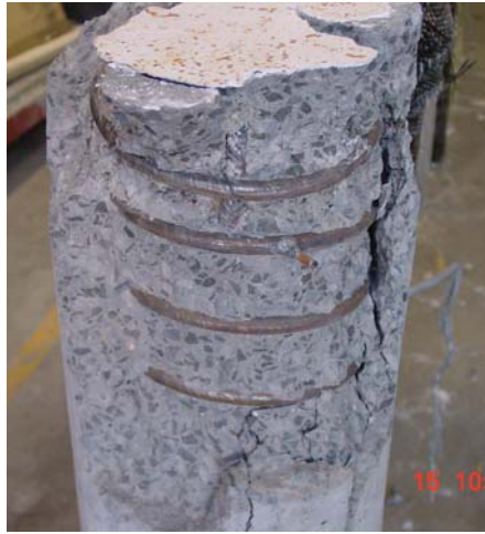
Figure 2 – Column N0 – Internal Reinforcement Only – e=0\text{mm}
