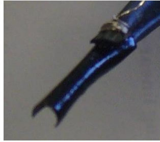
Fig. 9. Curling along the actuator.
