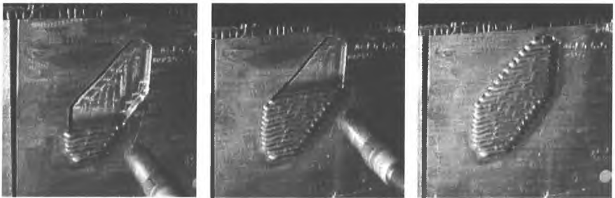
Figure 6. Deposit weld metal
