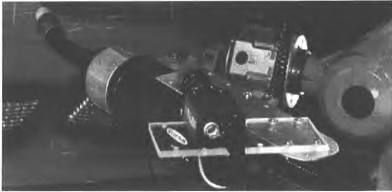
Figure 5. Touch sensing to determine workpiece profile
