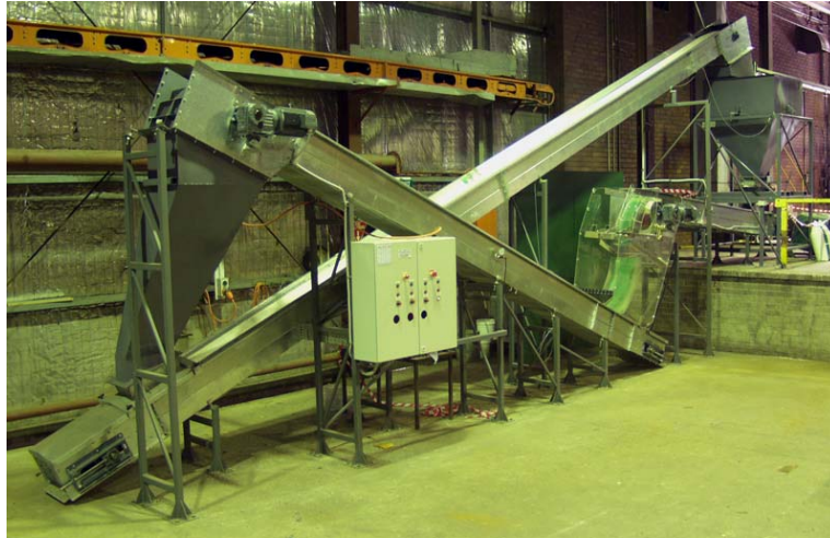
Figure 1 Conveyor transfer research facility
