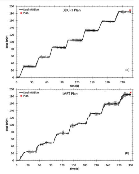
**Figure 5.** Real-time measured anterior rectal wall dose for (a) the 3DCRT plan and (b) the IMRT plan. The error bars are the 95% confidence interval of the average of three measurements.
