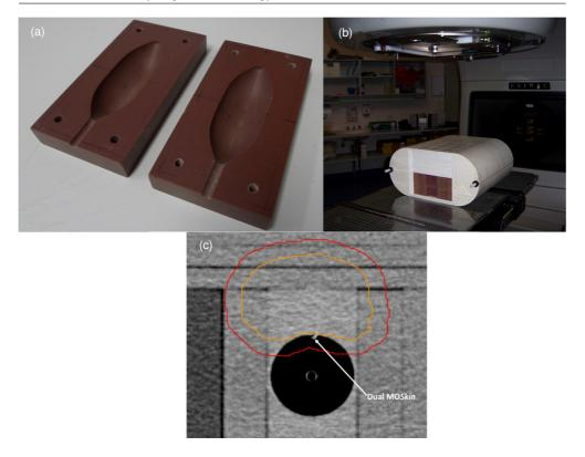
**Figure 2.** (a) Custom-made phantom to house the rectal balloon, (b) balloon phantom placed inside the IMRT phantom and (c) CT slice of the phantom showing the dual MOSFET location relative to the hypothetical prostate (inner contour) and PTV (outer contour).
