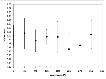
**Figure 4.** Dual MOSFET dose relative to the ion chamber measured dose at the centre of the IMRT phantom for a range of beam angles. The error bars are two standard deviations of the average of three measurements.
