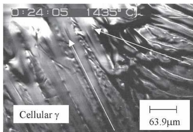
Fig. 9—Morphology of the austenite that has grown into the liquid phase in Figure 8. The arrows highlight the growth direction of two separate γ grains indicating there were two distinct nucleation events at the L/δ interface.
