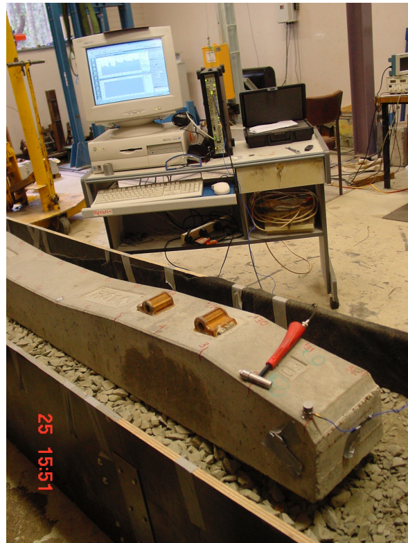
Figure 4. Experimental setup of a voided railway concrete sleeper
