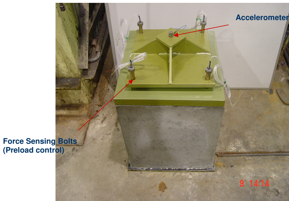
Figure 3 Innovative rail pad tester
