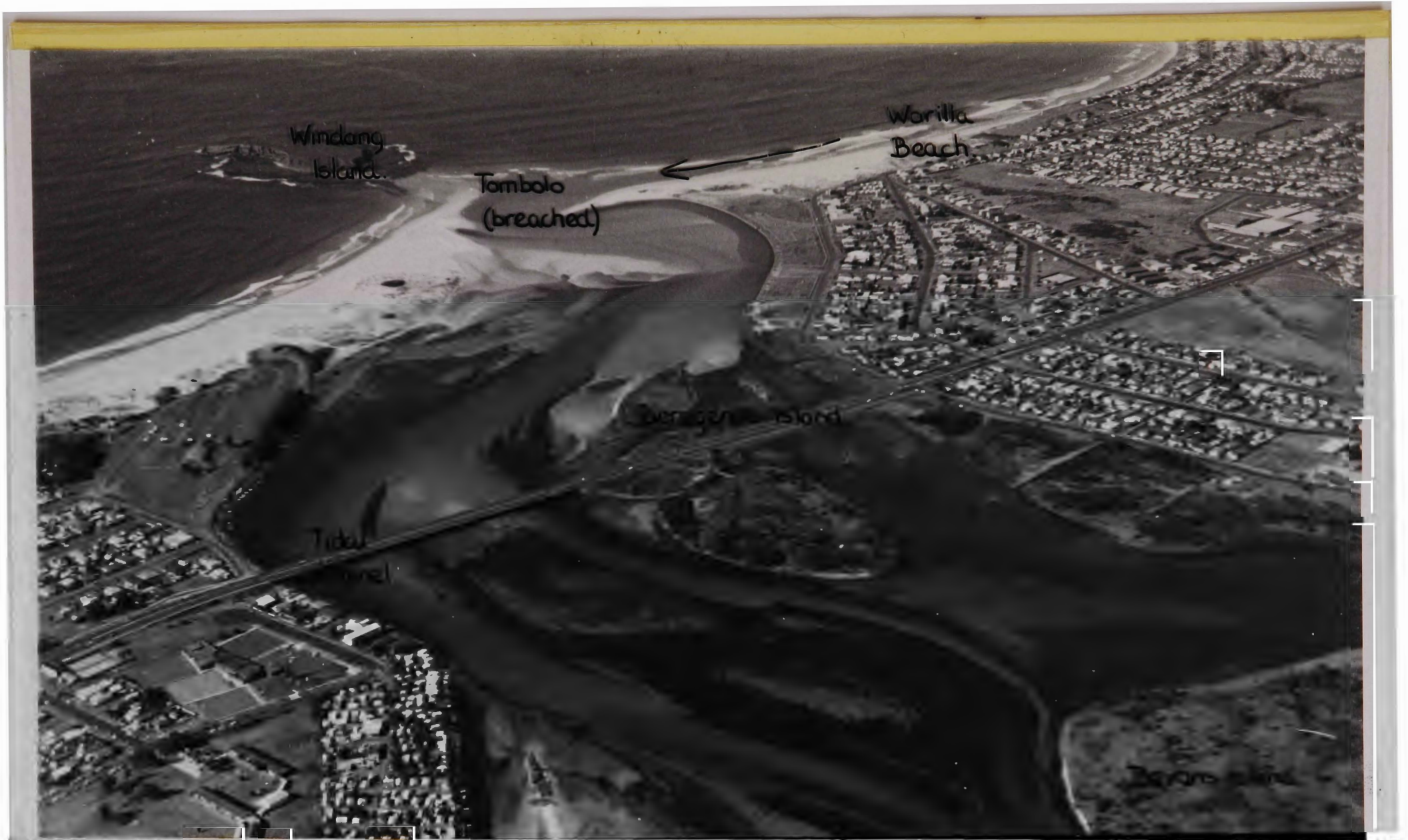
PLATE 1. Lake Illawarra entrance - The "Trap Door" Effect. Heavy seas breach the tombolo attaching Windang Island to the southern side of the lake entrance. South to north longshore drift may then transport sand from Warilla Beach into the lake entrance or onto Perkins Beach. The sand deposited in the lake entrance is gradually pushed up the tidal channel. When high seas subside, the tombolo reforms terminating the longshore drift and preventing compensatory southerly drift of sediment.
