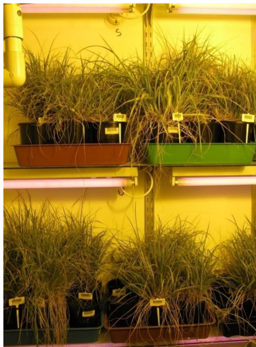
Figure 2.4 Planted and unplanted replicates in grouped SAB concentration trays within the growth room.
