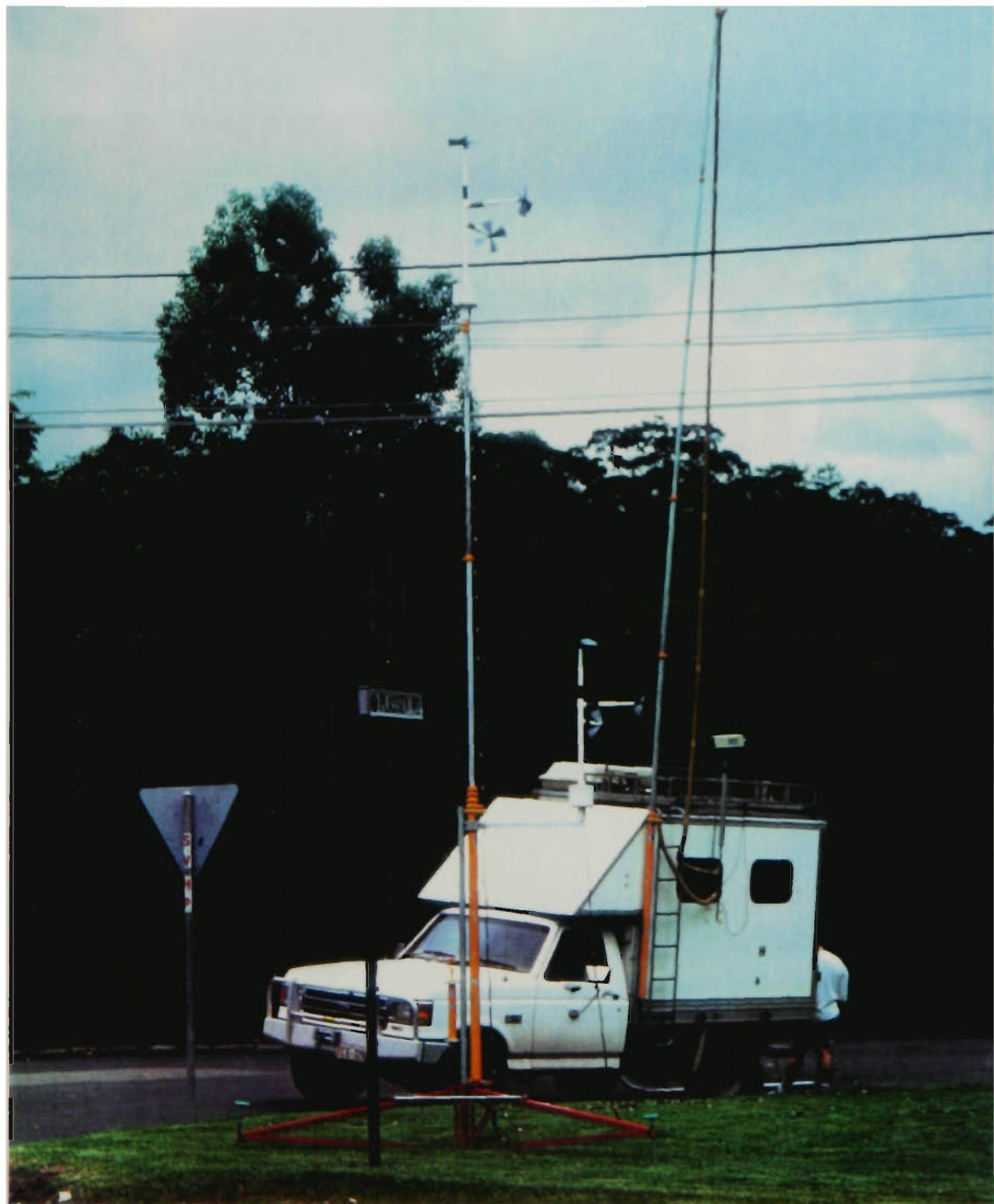
Figure 6.2 An overview for CSIRO instrumented vehicle with the anemometers and the two sampling lines (the fixed sampling line and the movable one).
