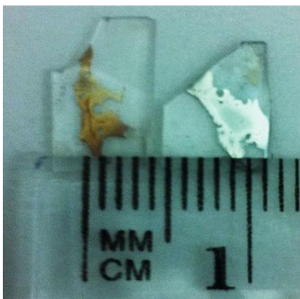
Figure 4-10: Optical image of two PDMS substrates coated with films of gold (left) and platinum (right). 5 \mu\text{L} of 10 % (wt) metal precursor solutions in ethylene glycol were dropcast on PDMS and the films were subsequently \text{N}_2 plasma treated for 5 minutes to reduce the precursor solution to metal.
