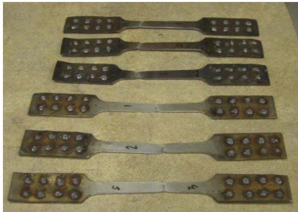
Figure 5.18: Tensile fracture of mild steel and stainless steel coupons.
