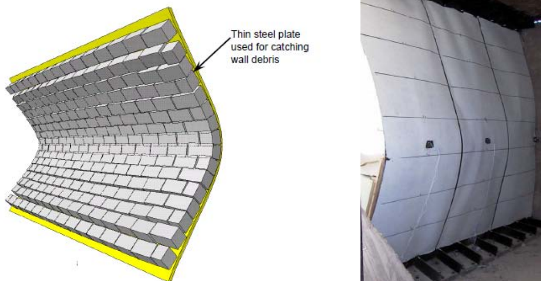
Figure 9.1: Masonry wall retrofitted by the thin steel sheet catcher system. (Crawford et al. 2009)
