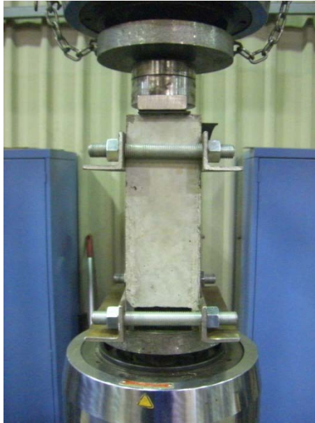
Figure 5.8: Push out test set up.
