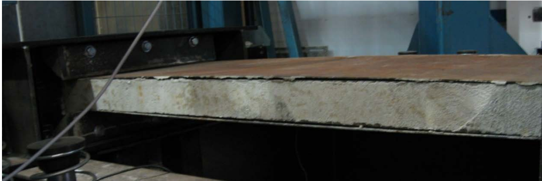
Figure 7.4: Separation of the steel faceplates from the concrete core for the Control panel prior to the impact test.
