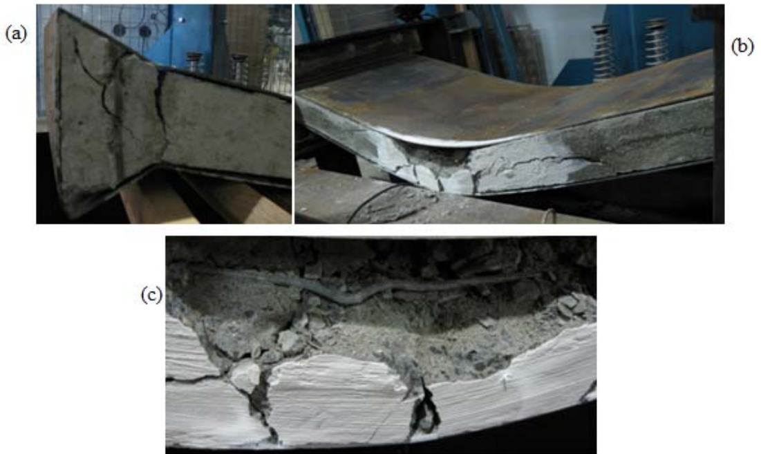
Figure 7.21: Damage on the Reinforced core panel: (a) cracking of concrete at flared zone, (b) crushing and cracking of concrete at mid-span, (c) buckling of top layer of wire mesh at mid-span.
