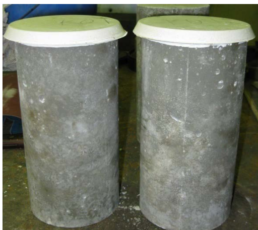
Figure 7.1: The concrete cylinders have been capped with high strength plaster before the unconfined concrete compressive test is conducted.
