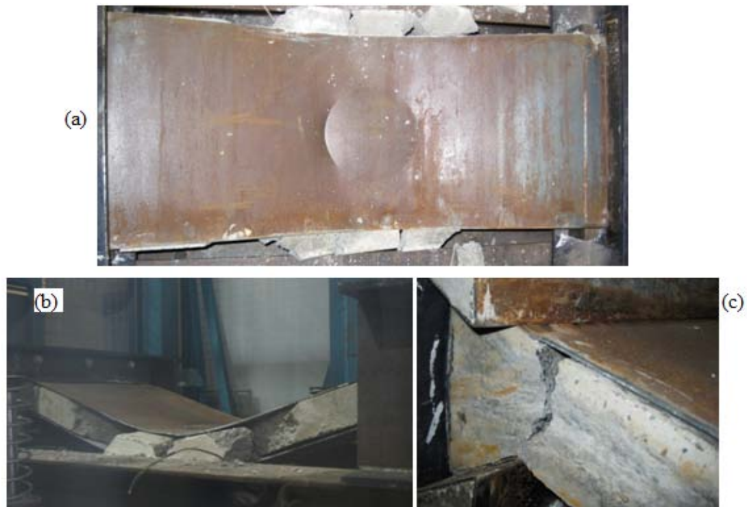
Figure 7.8: Damage on the Control panel observed after the impact test, (a) indentation on the top steel faceplate, (b) extensive damage of concrete core at mid-span, (c) wide crack at the support and buckling of steel end plate.
