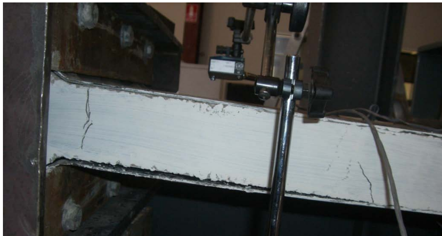
Figure 5.24: Separation of the bottom steel faceplate from the concrete core during the flexural response of the Control panel.
