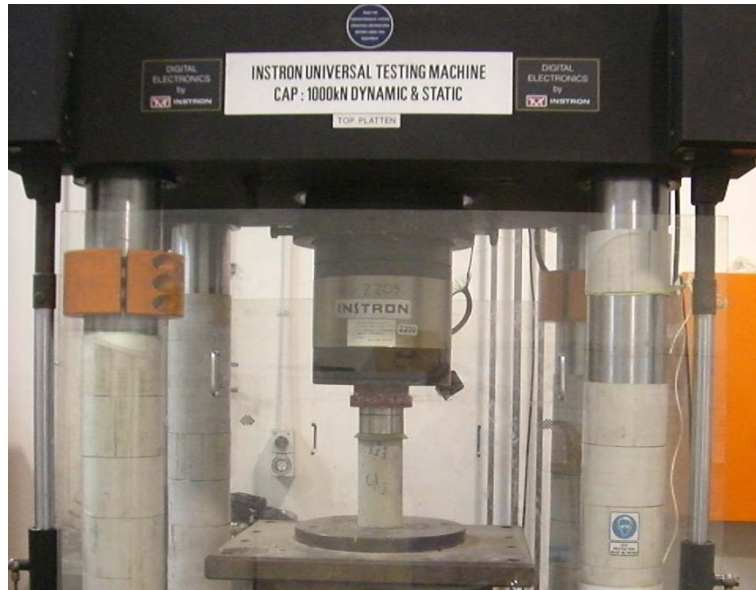
Figure 5.5: Unconfined concrete compressive test using the Instron Universal testing machine for normal weight concrete at the University of Western Sydney.
