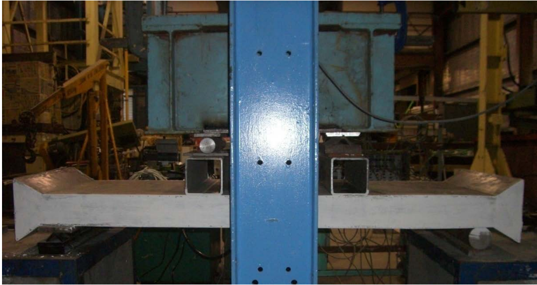
Figure 5.9: Experimental setup for a simply supported non-composite SCS panel under static four-point bending conducted at the University of Wollongong.
