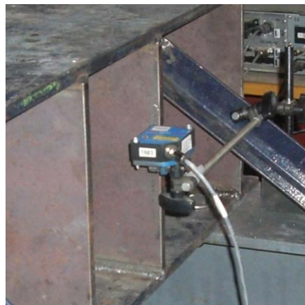
Figure 5.14: The laser displacement gauge used to record the displacement.
