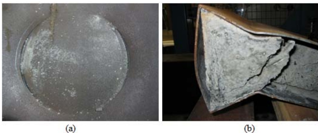
Figure 7.11: Damage on the Increased impact energy panel, (a) a partial fracture of the top faceplate, (b) buckling of the end plate.
