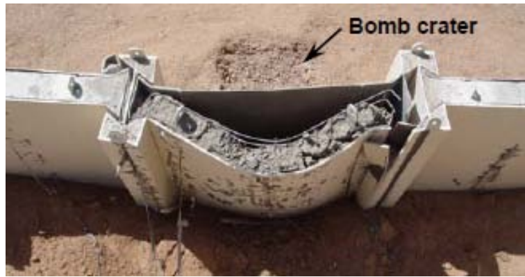
Figure 2.10: Deformation of Adler blast wall after subjected to close-in detonation of high explosive. (Crawford and Lan, 2006)
