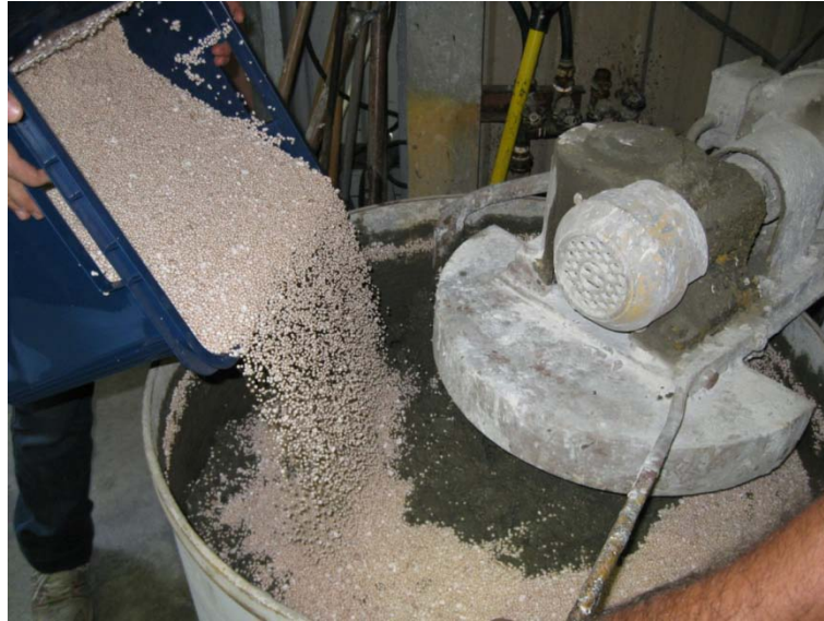
Figure 5.4: BST lightweight aggregates (polystyrene beads) being poured into concrete mix.
