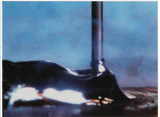
Figure 10.97 Pool at 400\mu\text{s} after short circuit for I_{\text{arc\_max}}=225\text{A}
