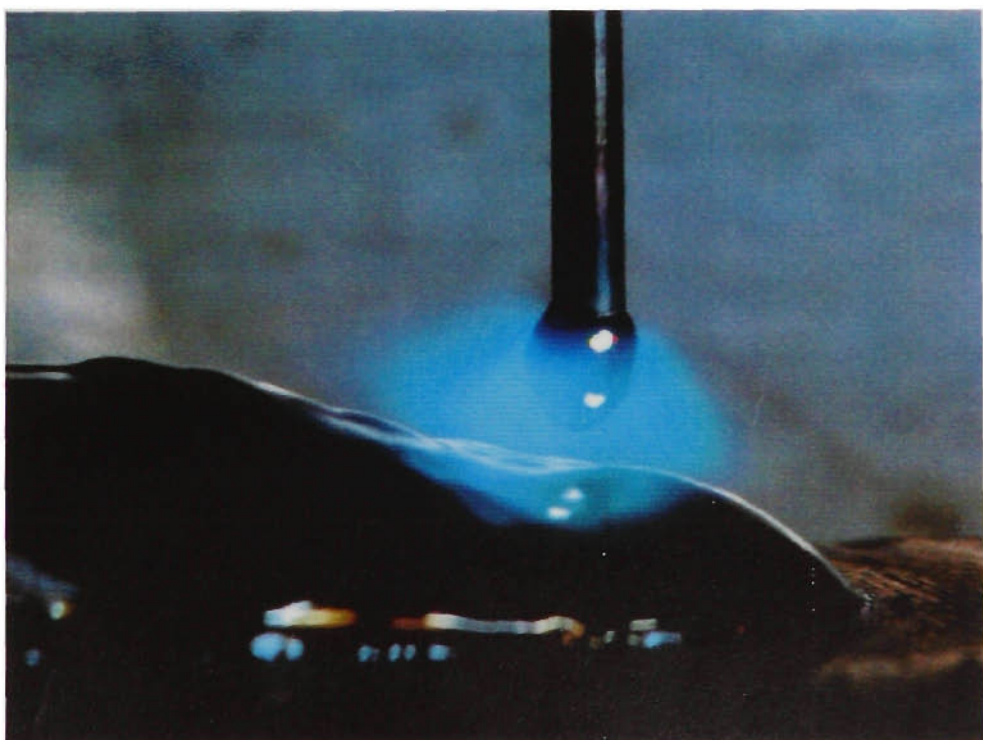
Figure 10.132 Pool depression in Ar-23%CO 2 , Iarc_min=100A
