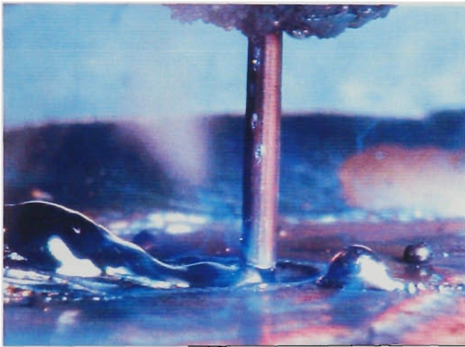
Figure 6.34 Photograph of short circuit with T_{sc} of 6.28ms
