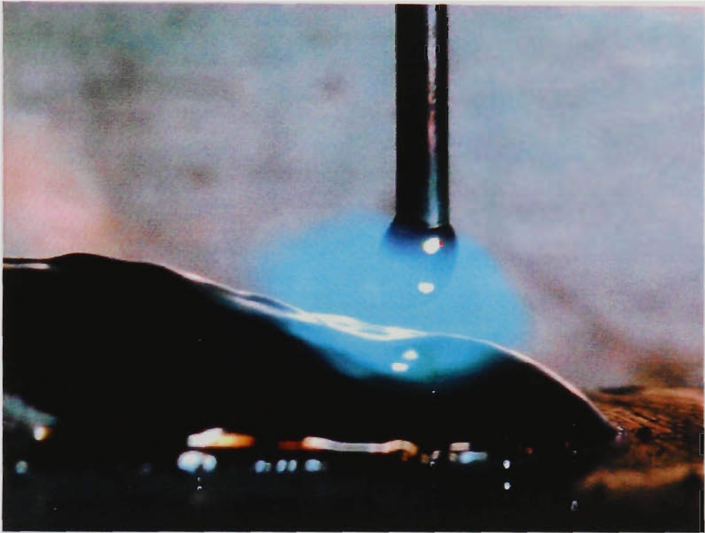
Figure 9.13 Photograph of arcing event at 100A
