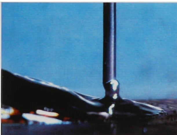
Figure 10.96 Pool at 400\mu\text{s} after short circuit for I_{\text{arc\_max}}=275\text{A}
