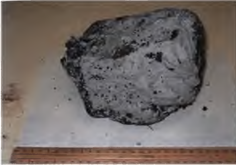
Plate 5.6: Excavated section of barrier (from preliminary injections)
