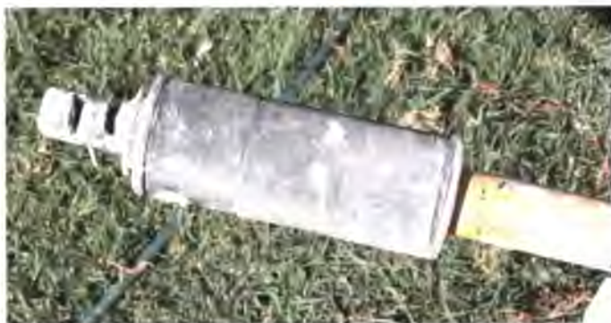
Plate 5.3: Modified tip of injection pipe.
