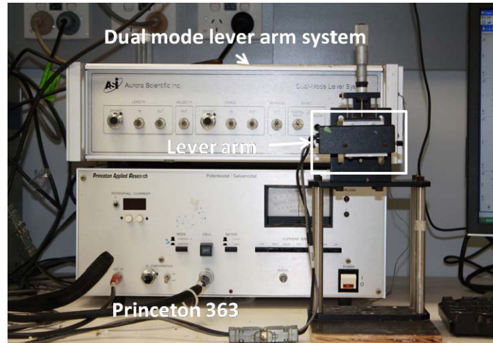
Figure 2. 9 Dual mode lever system for actuation test.
