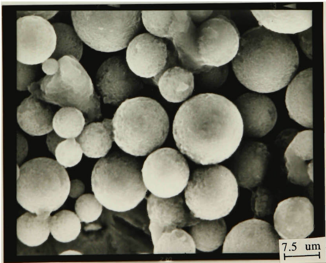
Figure 5.13: Scanning electron micrographs of sulfonate resin coated polypyrrole and polyaniline colloids. Conditions: (a 1 ) and (a 2 ) PVA, (b 1 ) and (b 2 ) PVP, (c 1 ) and (c 2 ) PEO stabilizer were used for the colloid preparation of polypyrrole and polyaniline respectively.
