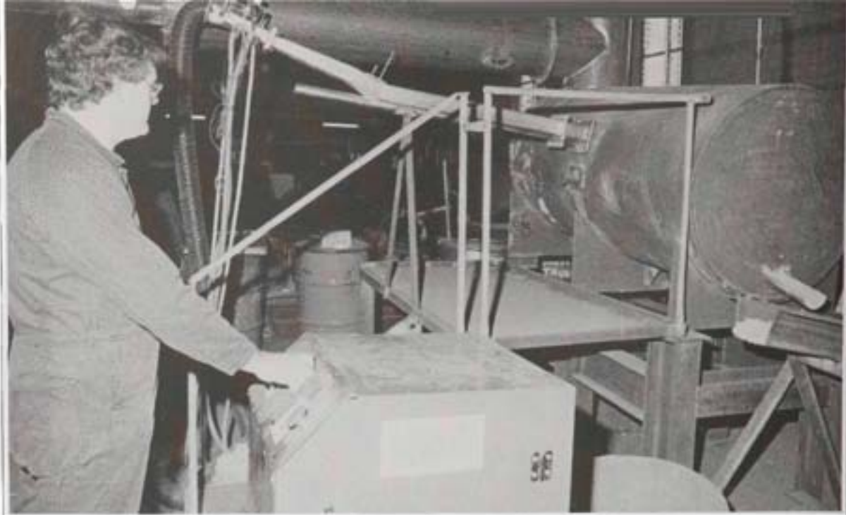
The University's research into the applications of microwave energy have led (and are leading) to many new and unexpected byways. At the research centre here is a pilot plant (one tonne/day) for the microwave smelting of tin from concentrate
