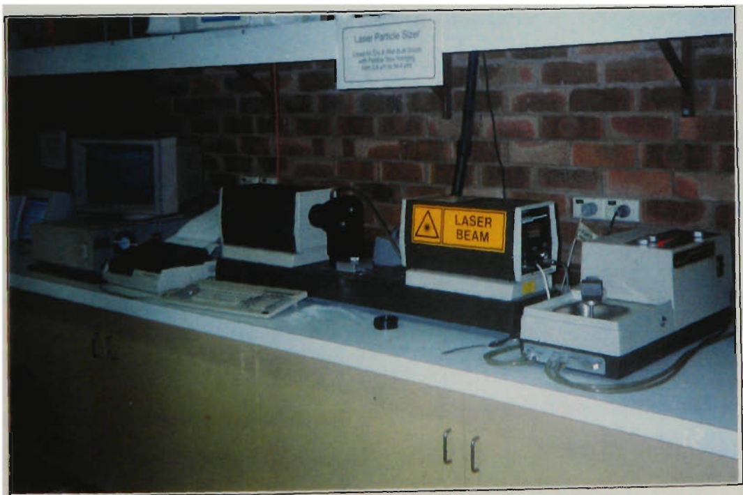
Figure 4.10 Model 2600 of Malvern laser particle sizer.
