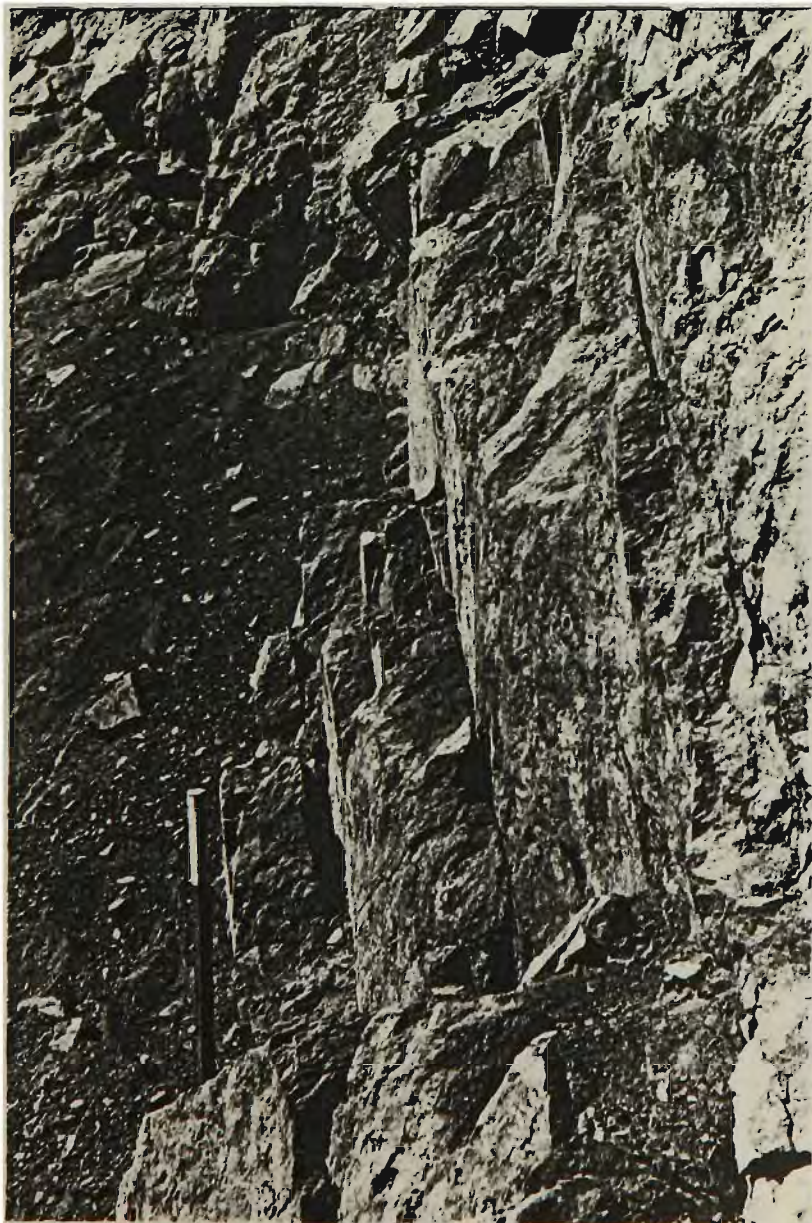
Plate 6.4 Planar shear jointing (set D) developed in the Beerina Dolerite A at approximately 7050E
