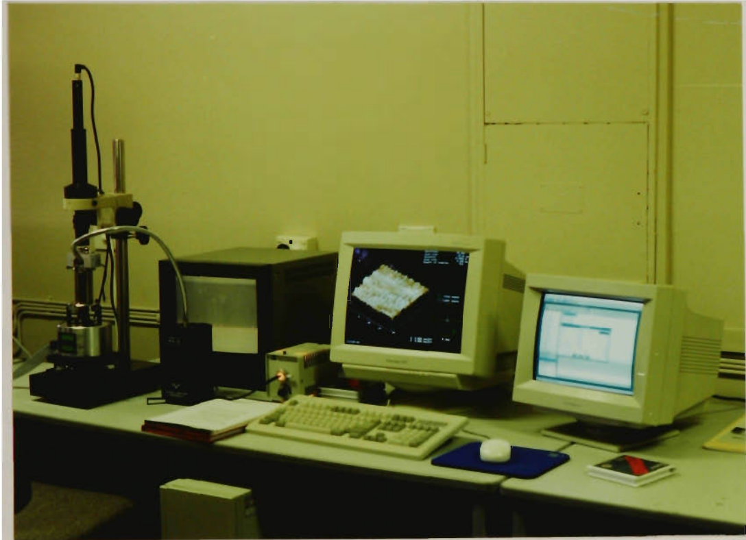
Figure 30. The NanoScope ® Atomic Force Microscope (AFM), from Digital Instruments, at the University of Wollongong.
