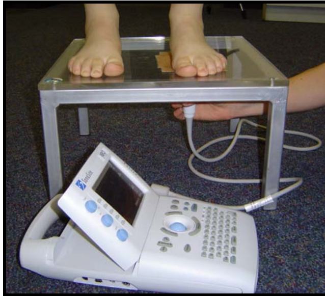
Figure 2. Experimental set up used to measure medial midfoot plantar fat pad thickness during weight-bearing.
