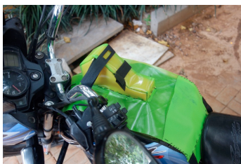
Figure 6: Rig for camera sensor module mount on the motorbike.
