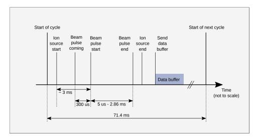
Figure 3.1: Example of the timeline of the events in the sequencer during normal operation.
