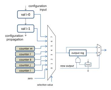
Figure 4.18: Circuit for output selection. The selection value is retrieved from the active microinstructions.
