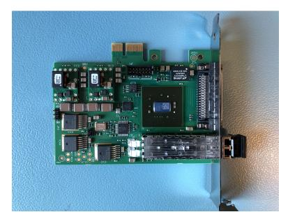
Figure 2.7: The PCIe-EVR-300DC card.
