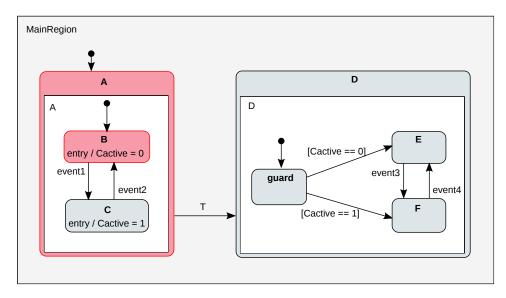
Figure 4.4: Statechart equivalent to the statechart shown in Figure 4.3 but without the forbidden transition.
