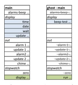
Figure 4.10: Main and ghost - main microprograms that implement the displays super-state. The microinstructions in the ghost microprogram replicate all the transitions taken by the main one, but they only perform actions when ghost - main runs the microinstructions that implement two specific AND-states: beep-taste and run. All other microinstructions are idle microinstructions and are struck-through.
