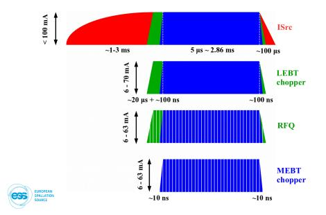
Figure 2.8: The beam pulse structure of ESS after several devices of the accelerator. Source: ESS.
