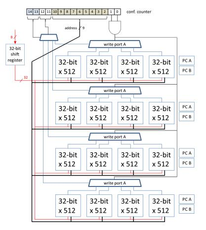
Figure 4.19: Load of a microprogram with four rows of four blocks per row. A simple configuration counter is used to load each word in the right position, row and memory block.
