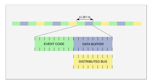
Figure 2.4: Frame structure of the data stream.
