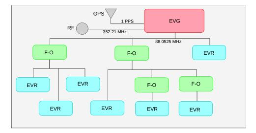
Figure 2.3: Topology example of the ESS timing system.
