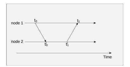
Figure 2.2: Calculating the delay of the transmission between two nodes.
