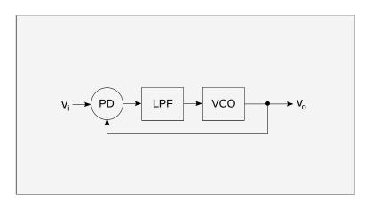
Figure 2.1: Phase locked loop.
