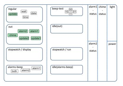
Figure 4.21: Example of microprogrammed organisation of states of the statechart in Figure 4.9. The dashed lines separate the AND-super-states. The leftmost one carries out most of the load, while its neighbour is mainly formed by ghost super-states with the exception of beep-test and stopwatch/run. The other five AND-super-states are very simple but, hierarchically, are at the same level as the main ones.
