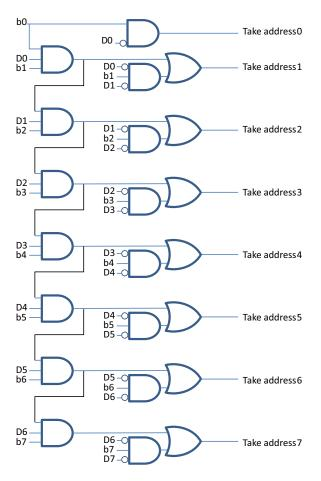
Figure 4.17: Example of chaining eight conditions. Eventually, all the conditions will activate only one output bit, which sets the transition that will take place.
