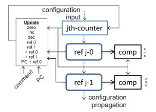
Figure 4.15: Scheme of a counter. At configuration time an initial and reference values are loaded. The counter behaviour is controlled by the active states.
