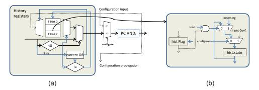
Figure 4.13: History register and its connection to the PC, which is updated when leaving the current OR-state. History is initialized at configuration time as shown in part (b) of the figure.
