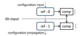
Figure 4.16: Input comparison. At configuration time two reference values are loaded. These values are used to calculate the current value with the reference ones during normal operation.
