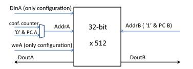
Figure 4.20: Dual port memory block. Two AND-states may be addressed simultaneously using both ports.
