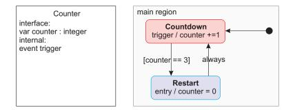
Figure 4.8: Simple statechart with actions and conditions.
