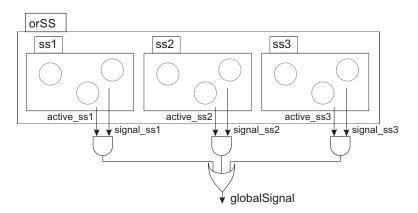
Figure 4.7: Distributed generation of a global signal.
