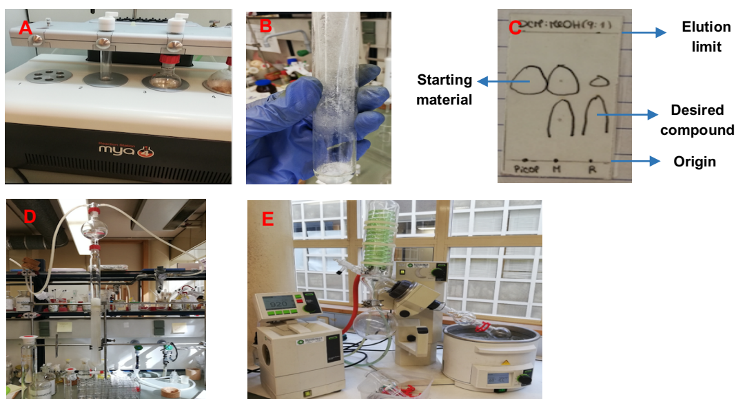
Figure 24. Pictures of the experiment process. (A) Mya4 reaction station. Temperature reaction was set to 130 °C for around 24 h; (B) Crude product ( [\text{C}_n\text{TPPBr}] ) outlook; (C) TLC plate of crude product ( [\text{C}_n\text{mPyrBr}] ) using dichloromethane:methanol (9:1) as mobile phase; (D) [\text{C}_n\text{TPPBr}] column chromatography by elution with the mixture of dichloromethane:methanol (9:1); (E) Solvent removal using a rotary evaporator.
