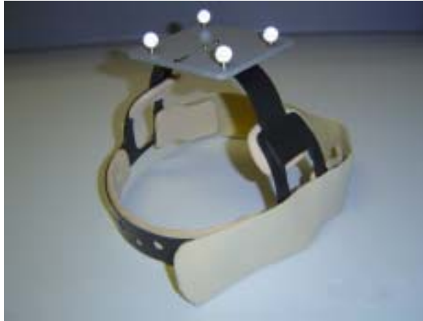
Figure 6.3. Head target attachment mechanism for the fourth volunteer. The semi-rigid plastic strap that formerly passed across the back of the head was cut away and replaced with a soft strap fastened using Velcro ® . This modification was aimed at minimising ‘catching’ of the device on the patient bed and thereby minimising the decoupling of target and head motion.
