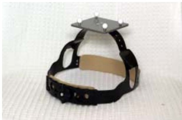
Figure 6.1. Modified welding mask used to attach the head target (grey slab with spherical reflectors) to the patient head. There are three semi-rigid plastic straps: one passing across the forehead, one across the back of the head, and one across the crown of the head. The target is secured to the top of the crown strap.
