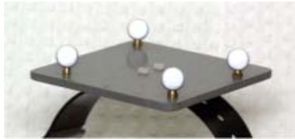
Figure 5.1a. The head target. Four infrared-reflective spheres were attached to a 3mm square slab of polyethylene to form this target.
