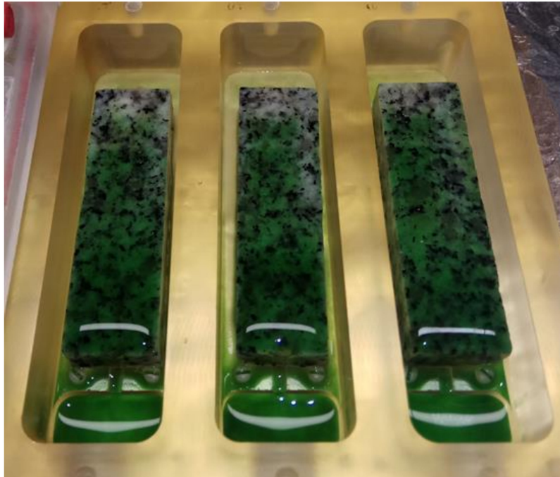
Figure 1. Biofilms formed on granite samples after incubation for 21 days in a drip flow reactor with carbon-enriched medium.
