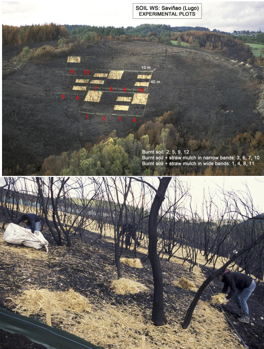
Figure 5 and 6: View of the macro-plots in the area affected by a wildfire. (12 experimental plots, 10 × 40 m each), and detail of straw mulch application. Treatments: B, burned soil (2, 5, 9, 12); B1S+M, treatment with 1 straw strip per plot, soil with straw mulching; B1S, treatment with 1 straw strip per plot, bare soil (1, 4, 8, 11); B2S+M, treatment with 2 straw strips per plot, soil with straw mulching; B2S, treatment with 2 straw strips per plot, bare soil (3, 6, 7, 10). (Author: Serafin Prieto González).
