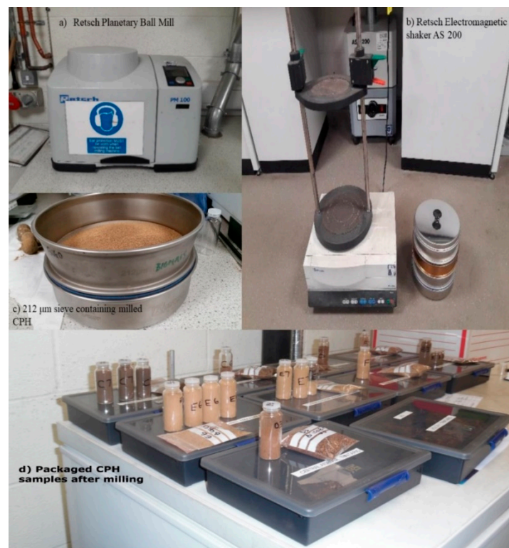
Figure 3. (a) Retsch Planetary Ball Mill PM 100. (b) Retsch Electromagnetic Shaker AS 200. (c) Sieve containing milled CPH. (d) Packaged CPH sample after milling.
