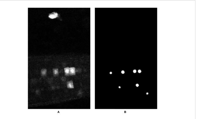
FIGURE 9 | Representation of the output volume (B) for input data (A) produced by the network trained on the re-shuffled dataset, featuring a wider variety of training data. Note the artefact outside the root, at the top of the image, is no longer labelled on the output.
