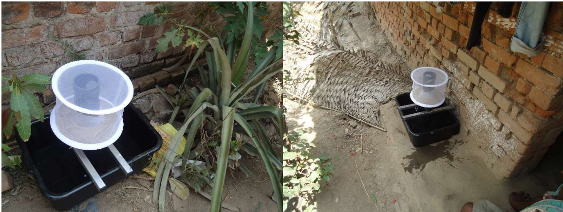
Figure 5.3. CDC gravid traps in location at houses used to collect of mosquitoes, in particular gravid female Cx. quinquefasciatus .
