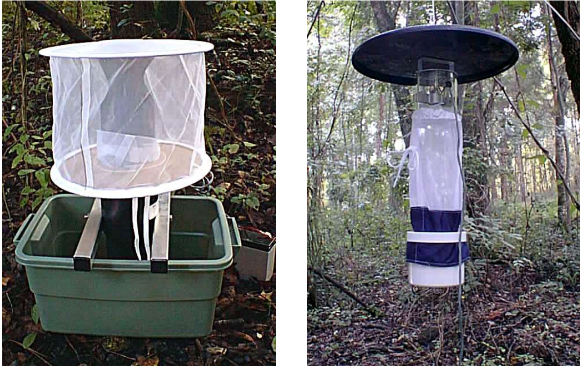
Figure 4.2. Showing a CDC gravid trap (left) and a CDC light trap (right). Image courtesy of http://www.johnwhock.com/
