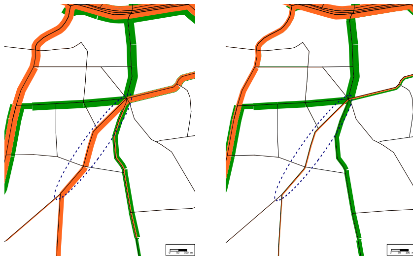
Fig. 9: Parts of the Halle network model before (left) and after (right) the most successful run of the local optimisation experiments. Links are displayed in black and the link loads are displayed by orange bars (PrT load in terms of number of vehicles) and green bars (PuT load in terms of number of passengers) along the links. The thickness of the bars indicates the relative volume of the load. The dashed blue circle marks the links selected for optimisation.
