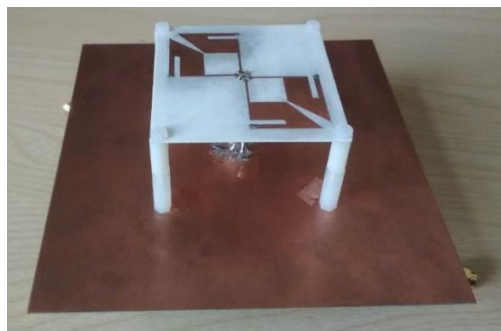
Figure 4.11 Photograph of the fabricated prototype of the proposed differentially driven dual-polarized antenna.
