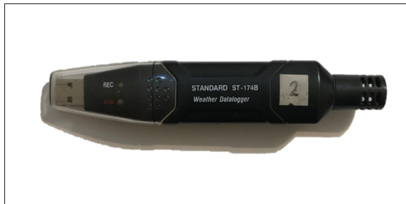
Figure B1. Standard ST-174B weather datalogger for measuring T_A to validate ENVI-met.
