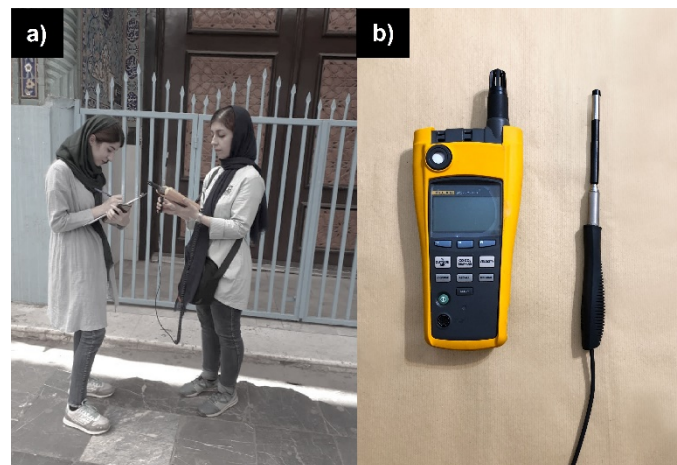
Figure 3.a) Micrometeorological measurements simultaneously with the completion of the questionnaire in the study site. b) Fluke 975 sensor for measuring T_a , RH, and WS.
