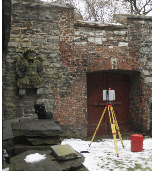
Figure 1-1: Laser scanner used for the 3D recording of Sint-Baafs Abbey (Ghent, Belgium)
