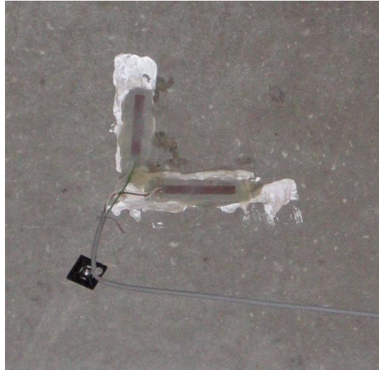
Figure 5-5: Strain gauge installation on the concrete surface
