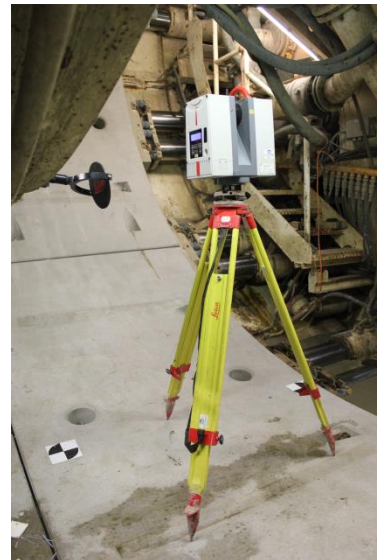
Figure 4-2: Three scanning positions for a reference measurement (left); Third scanning position during a reference measurement in the TBM (right)
