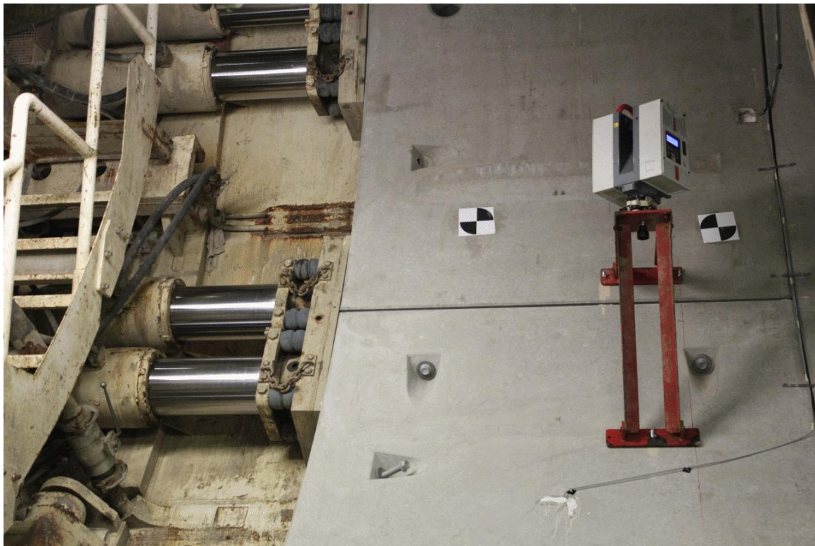
Figure 3-3: Laser scanner mounted on a bracket at one side of a tunnel section
