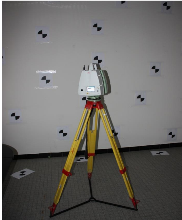
Figure 9-1: Setup of a laser scanner Leica C10 for a user self-calibration measurement
