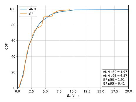
**Figure 10.** Cumulative distribution of the error evaluated on set *A* for the Machine Learning (ML) methods in the case the absolute intensities *r* are used as features.
