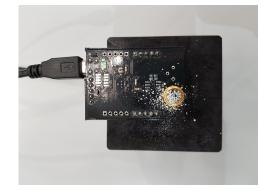
(a) The receiver aperture obscured by white chalk dust, this corresponds with the measurements in dataset *D*.
