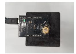
(**b**) The receiver aperture obscured by saw dust, this corresponds with the measurements in dataset *E*.
