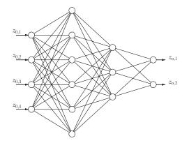
**Figure 1.** Structure of an Artificial Neural Network (ANN), which consists of multiple nonlinear transformations  $\sigma(W_i z_{i-1})$  of the inputs  $z_0$ .
