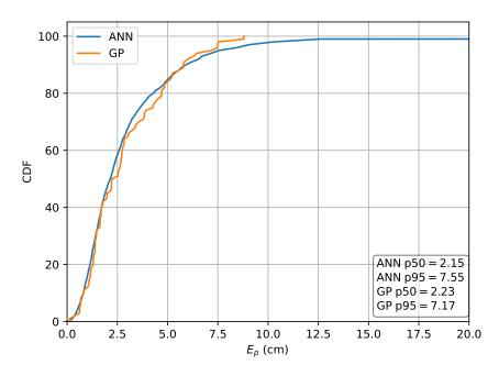
**Figure 12.** Cumulative distribution of the error evaluated on set *A* for the ML methods in the case the relative intensities  $r_{rel,all}$  are used as features.
