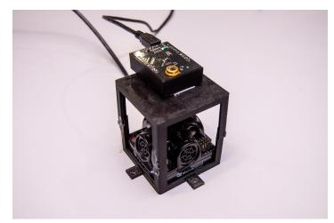
**Figure 6.** Image of the custom designed receiver in the experimental setup, the device on the top is the Visible Light Positioning (VLP) receiver and the device on the bottom is the mobile node of the acoustic ground truth system (Marvelmind Robotics Super-NIA-3D).
