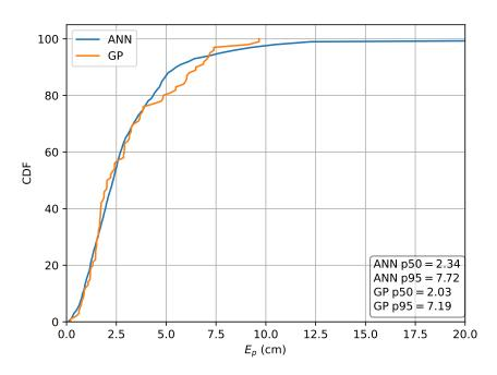
**Figure 11.** Cumulative distribution of the error evaluated on set *A* for the ML methods in the case the relative intensities  $r_{rel,max}$  are used as features.
