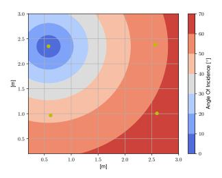
**Figure 5.** A top view of the set-up with the angles of incidence  $\gamma_l$  at the photodiode (PD) highlighted for a single LED. The wide range of angles of incidence results in a representative experimental set-up.
