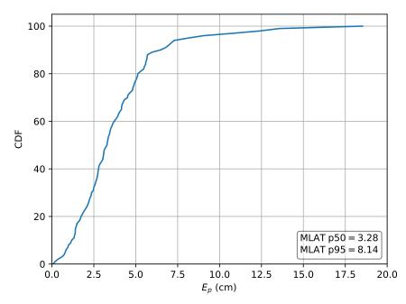
**Figure 13.** Cumulative distribution of the error evaluated on set *A* for the absolute multilateration scheme using *r* as input.
