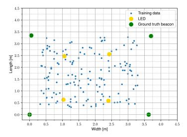
**Figure 4.** A conceptual top view of the setup with four LEDs at a height *h*. The measured data from the experimental set-up is sampled randomly in the receiver plane.
