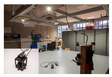
**Figure 3.** A photo of the complete experimental set-up with four light-emitting diodes (LEDs) at height h = 1.284 m.
