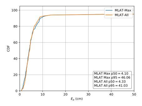
**Figure 14.** Cumulative distribution of the error evaluated on set *A* for the relative multilateration schemes using  $r_{rel,max}$  and  $r_{rel,all}$ .
