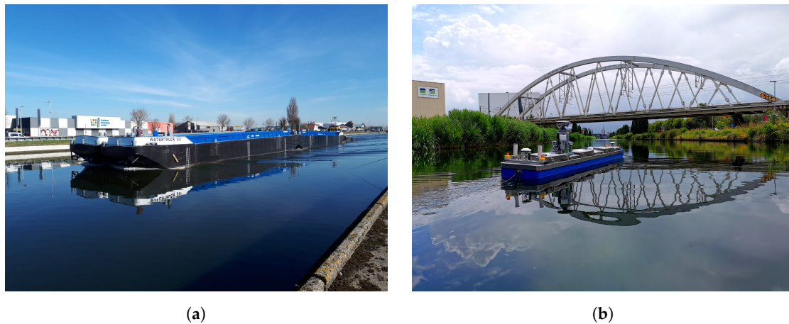
Figure 1. The Watertruck + concept: (a) four full-sized barges pushed by a push boat [1], reproduced from [4] with permission from MDPI, 2020; (b) the KU Leuven scale model of a self-propelled barge named Cogge [3].
