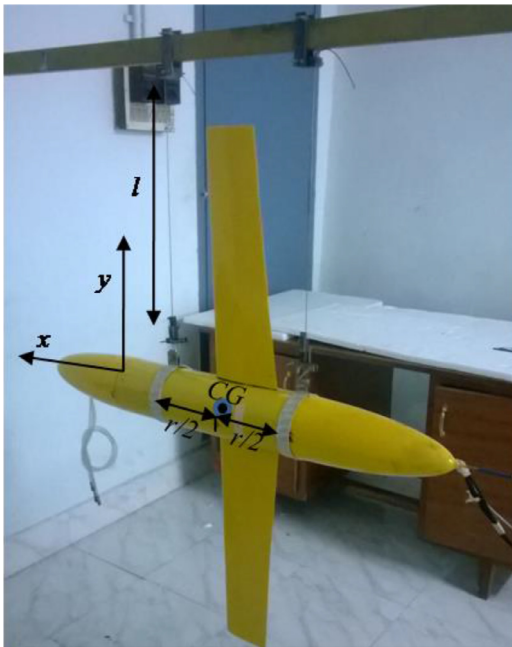
Fig. 44. Test set up for determination of I_{yy} .
