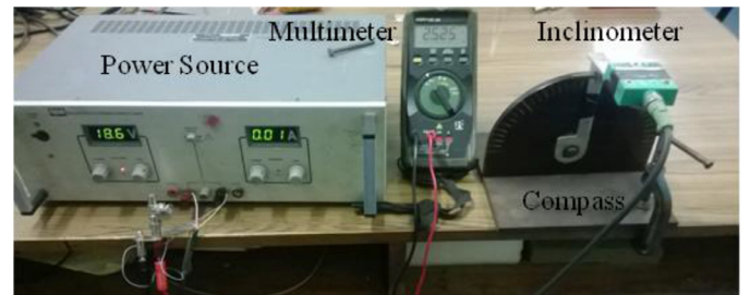
Fig. 51. Setup for calibration of inclinometer.
