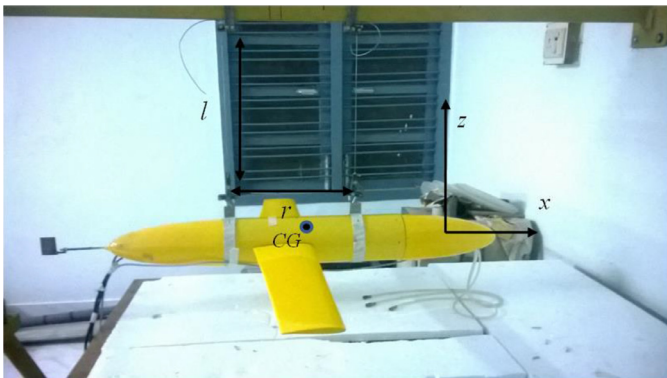
Fig. 40. Test set up for determination of I_{zz} .
