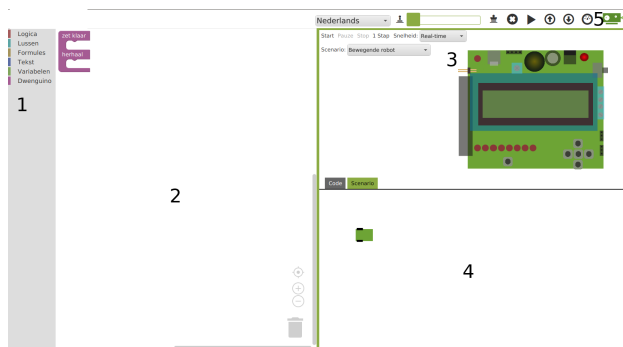
Fig. 2: Overview of the custom programming environment. (1) The toolbox repository with all the blocks that can be used. (2) The workspace area, this is where programs are constructed. (3) The microcontroller board simulation. (4) A simulation of a riding robot similar to the one they build during the sessions. (5) Controls for saving, restoring and uploading the code to the microcontroller board
