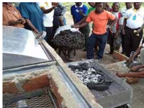
FIGURE 36 Participants using charcoal to smoke fish on FTT kilns installed in their community in the United Republic of Tanzania
