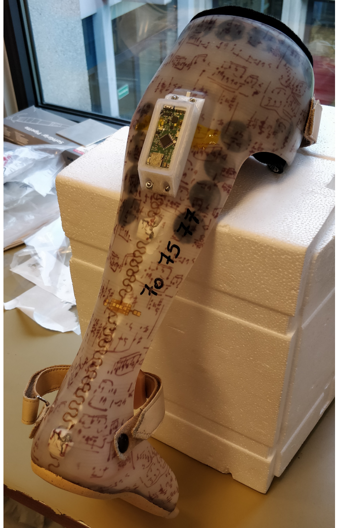
Fig. 5. A finalized I2AFO. Three embedded IMUs are read out by an external central microcontroller, which transmits the sensor data wirelessly through Bluetooth.
