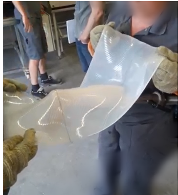
Fig. 2. The heated PP sheet is thermoformed by draping it over a designed mold.
