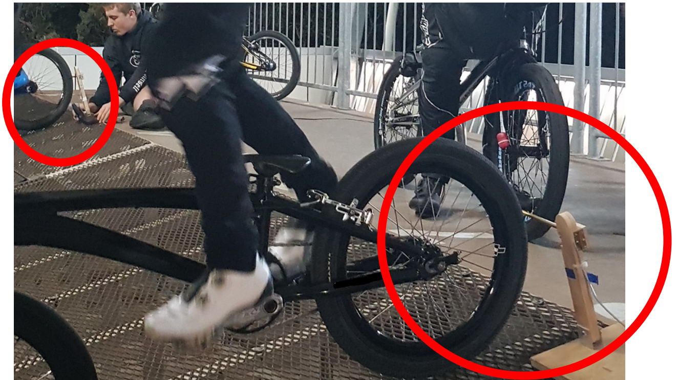
Figure 6-7 Reaction timer setup on the SX ramp.
