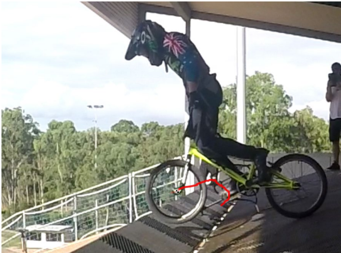
Figure 8-6 The hub trajectory is traced in red from the starting position in Kinovea.
