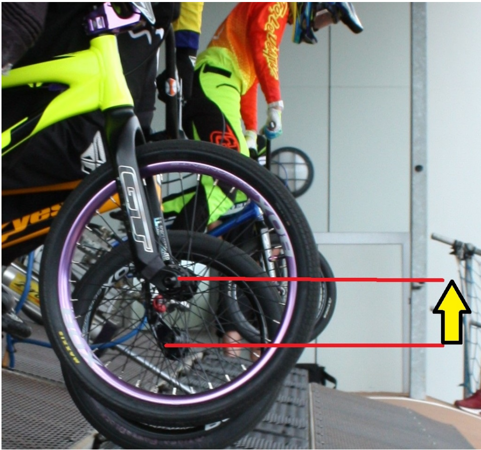
Figure 8-4 This figure shows the front hub at its maximum height. The hub lift is measured as the distance from the start height to the highest point on the hub trajectory.
