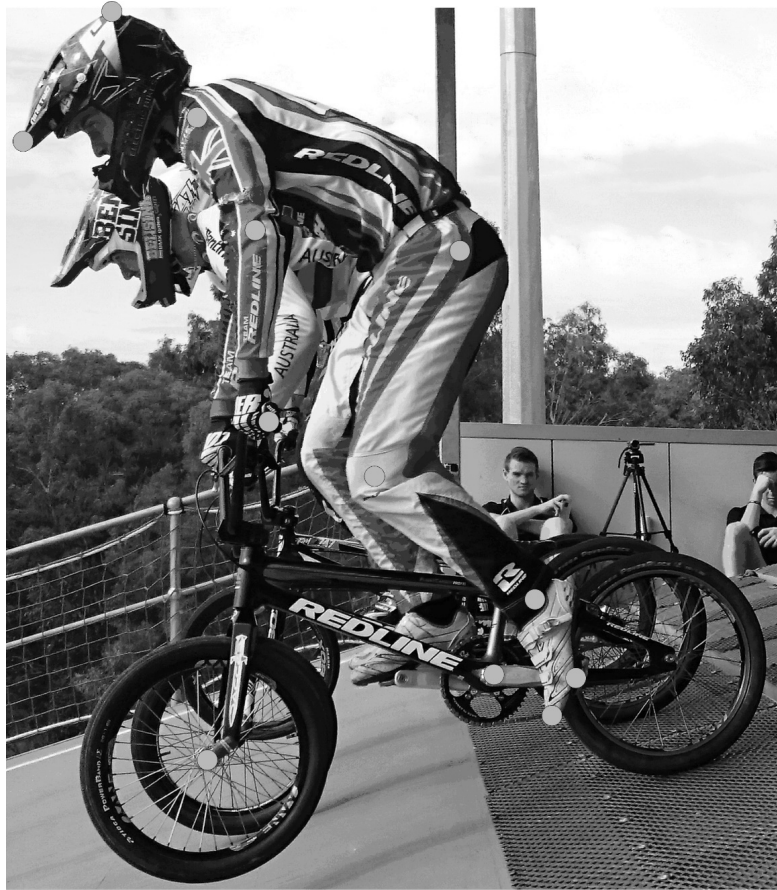
Figure 7-4 Virtual markers are added to the figure and tracked through 150 frames. Markers are added to the front of the helmet, rear of the helmet, front hub, handlebar end, elbow, shoulder, hip, knee, ankle, toe, crank centre and crank end.
