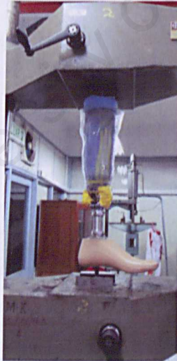
Figure 3. Tensile testing for the new prosthesis coupling system.
