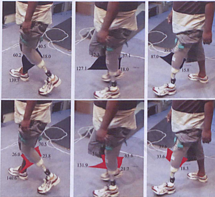
Figure 8. Pressure profile with new magnetic lock (top) and pin/lock systems (bottom) during stance; right to left: early stance, mid stance, late stance. All values (average peak pressure) are in kPa.
