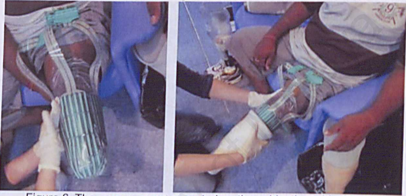
Figure 6. The sensor arrays mounted on the subject's residual limb.
