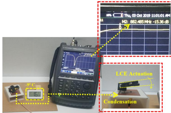
Figure 6.40. The LCE array is actuated at -9^{\circ}\text{C} . The switch has been triggered and the operating frequency of the antenna design is 882 MHz
