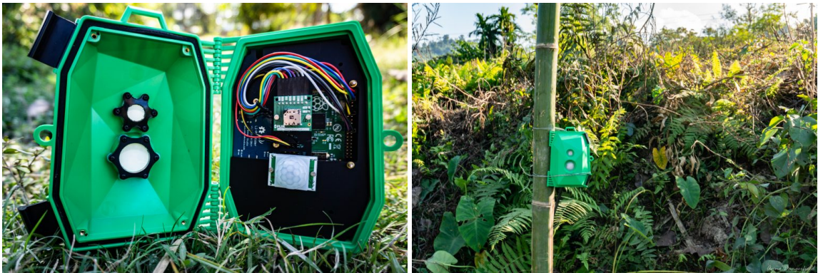
Figure 3.1: Camera trap used in Assam, India. Image source: Arribada Initiative [13]
